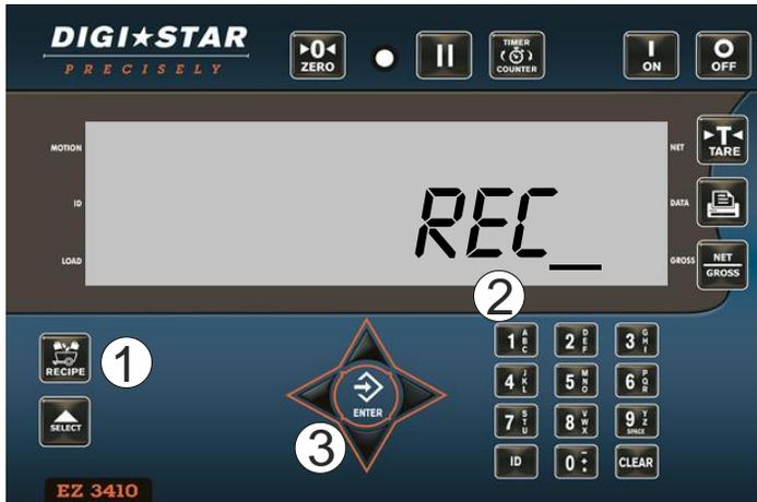
1. Press and hold
