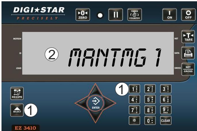
1. Enter D.A.N. 8011 then press
