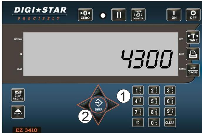
1. Enter desired preset weight using key pad.
