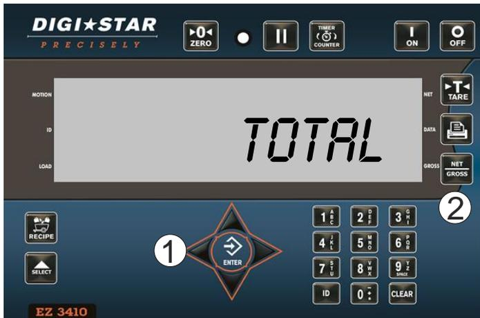
1. Press and hold arrow to erase the current ingredient or pen displayed on the screen.
