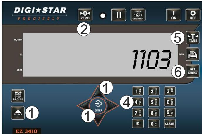
1. Enter 1103, press . Press UP arrow or to enable this feature. Then press to return to weighing mode.
