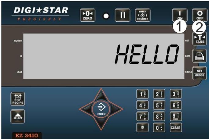
1. Press **ON** to turn indicator on. Indicator will turn on and display "HELLO", a message may follow, and indicator will then display a number for the weight in the bin.
