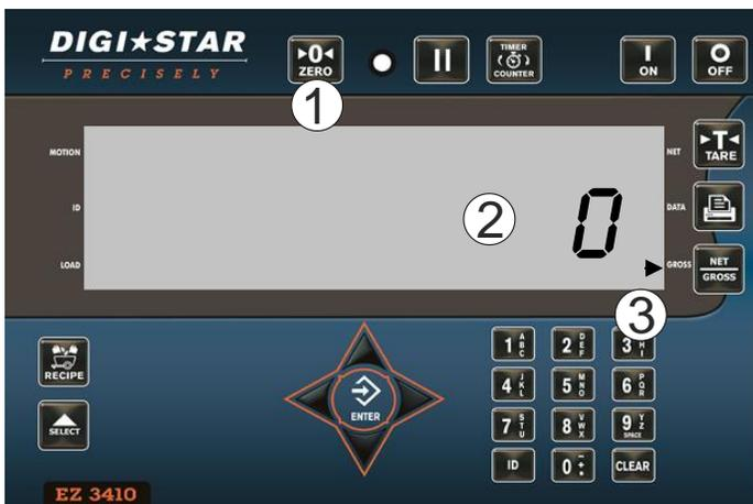
1. Press and hold **ZERO** for three seconds to zero balance scale.
