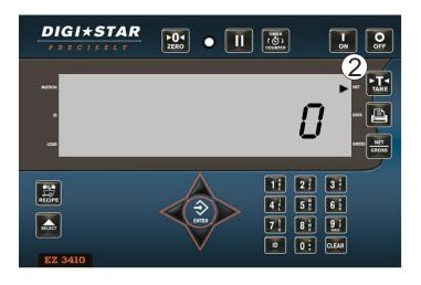
2. Press to set weight to zero. Flashing arrow points to net.
