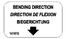
Observe direction of arrow when installing load cell.
