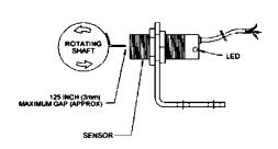
Use with EZ3410 indicator. Sensor allows operator to program indicator to count auger or PTO rotations for accurate mixing of feed. Also used for keeping maintenance log for equipment. Example; At 50 hours of operation time PTO shaft is scheduled for greasing or engine oil is scheduled for changing. For proper equipment maintenance needed, refer to equipment operator manual.
