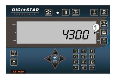
1. Press to send data to printer or PC. Flashing arrow on side of display points to DATA.
