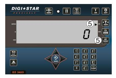
5. Pressing again shows the net weight of 300. In Net mode flashing arrow points to NET.
