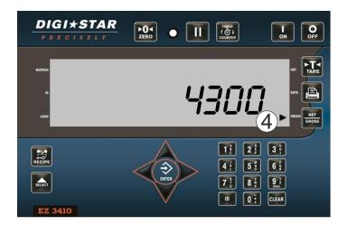
4. To show total of original weight of 4000 plus added 300, press flashing arrow on side of display points to GROSS.
